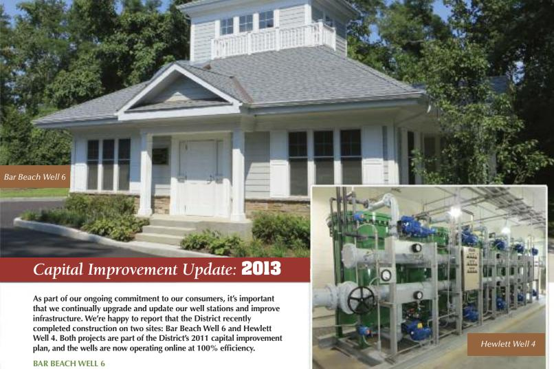
A new Packed Tower Aeration System has been constructed at the Bar Beach Well 6 site for the removal of Volatile Organic Contaminants (VOCs) detected in the raw water. To remediate the issue, the District took the well offline in 2011, thereby designating the completion of this project as high priority. Built from the ground up, the plan included a full architectural residential design of the building and landscaping features to help the new facility blend into the community.
